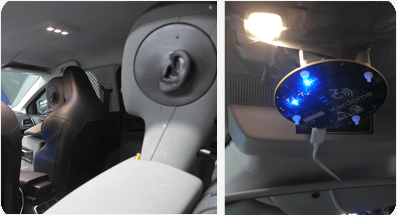
Fig 1: Evaluation setup with four Artificial Head Measurement Systems and Kardome's Gavel Evaluation Kit.
