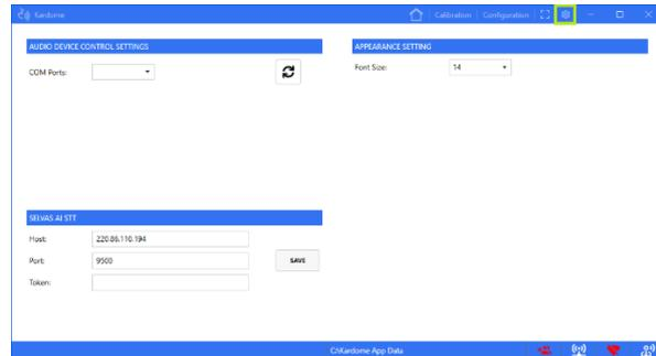
2. Select the appropriate COM Port to which the Mallet card is connected. If the port is not in the list, press on the refresh (🔄) button.
