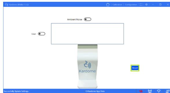
3. Calibrate the initial ambient noise characteristic by activating the *Ambient Noise* switch and wait until the process is completed. Upon completion, the switch turns to blue.
