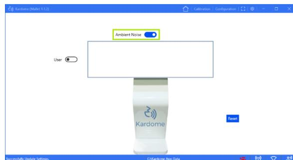
4. Calibrate the initial user acoustic signature by activating the *User* switch and wait until the process is completed. Upon completion, the switch turns to blue.
