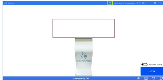
2. To use the Kardome algorithm turn on the 'Kardome Enable' button. If the button is turned off the Mallet will be used as a passive microphone array.
