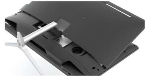
TOOL-LESS CHASSIS • Easy Repair
