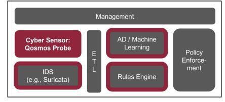
The Qosmos Probe provides essential data that complements IDS/IPS, feeds anomaly detection algorithms in the machine learning module, and enables the creation of advanced rules.
