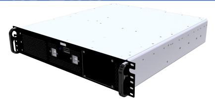
**Field-tested, fail-safe, and long-life performance in extreme conditions.** The IS2502 industrial server is designed for demanding applications that require high-performance computing and high-capacity data storage. Constructed with a rugged, all-aluminum chassis and state-of-the-art thermal management, this powerful, compact server delivers seamless performance in the most harsh, unpredictable environments. It also meets strict environmental emission standards for an eco-friendly solution.
