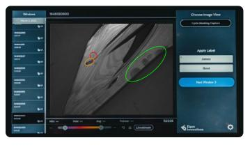
A screen at the paint line displays a view of the entire part surface and flags parts with common defects such as dirt, scratches and orange peel. It even detects finger prints.
