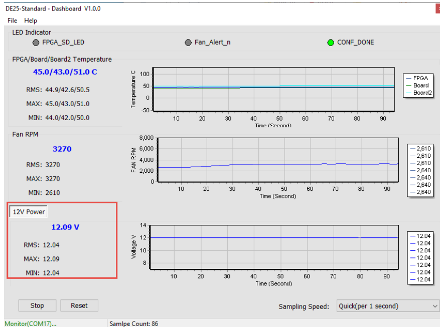
Figure 4-12 Power Monitor Section
