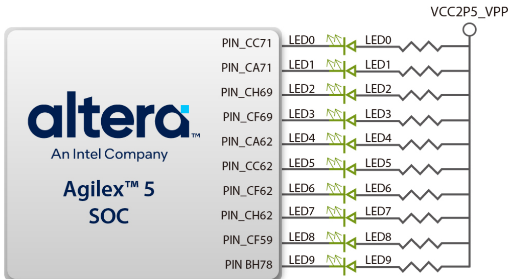
Figure 3-20 Connections between the LEDs and the Agilex 5 SoC FPGA
