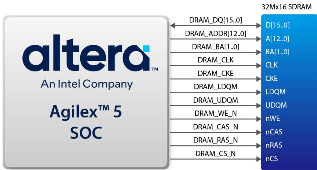
Figure 3-32 Connections between the FPGA and SDRAM
