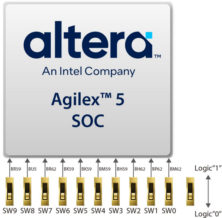
Figure 3-19 Connections between the slide switches and the Agilex 5 SoC FPGA
