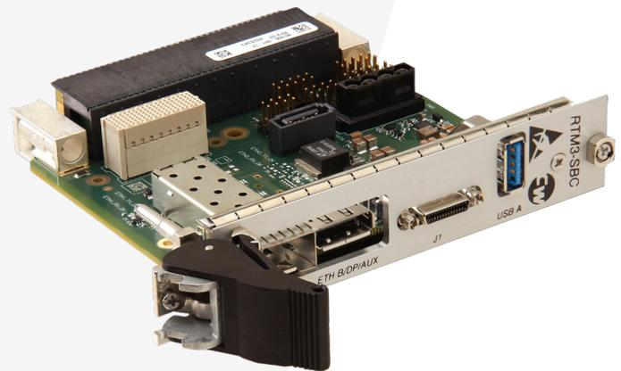
Figure 3: Rear Transition Module
