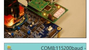
4 times a Byte to 80, 81, 82 and 83, and 2 times a Word to port 80 and 82 BIOS POST code example
