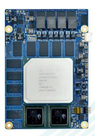
Intel Agilex 7 R24C SoC FPGA based System on Modules features Agilex F-Series R24C Package Family - AGF 006, AG 008, AGF 012, AGF 014, AGF 019, AGF 022, AGF 023, AGF 027 Supports a Hard Processor System comprising of Quad-core 64-bit ARM CortexA53 up to 1.4GHz.
