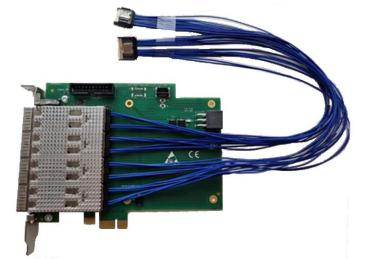
With the adaptor offered the ThunderFjord provide QSFP-DDs for 400GE along-side 4xQSFP28s for extra 4x100GE or 16x10/25GE via breakout cables ensuring additional Ethernet bandwidth and high port and speed flexibility.
